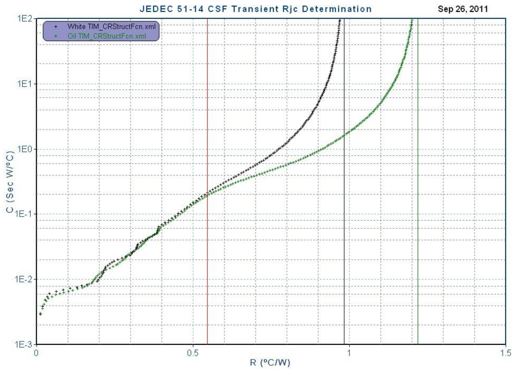
Figure 30: JEDEC 51-14 Rjc CSF comparisons for “White & Oil” TIMS
