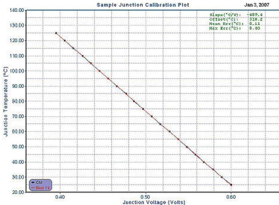
Once this junction calibration data is collected, the junction temperature of the device under test is computed as
